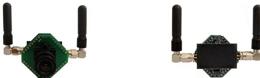
Figure 2.2: Prototype for Our Battery-Free Video Streaming Camera with Dual Power Harvester. The FPGA is located behind the solar cell.
