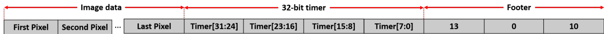
Figure 5.4: Packet structure of the dual camera sensor node. Each cell has a byte of data. Our sensors record the image data and add the timer value and footer to the end of the packet. Timer data and footer are used to synchronize the sensors with the laptop.
