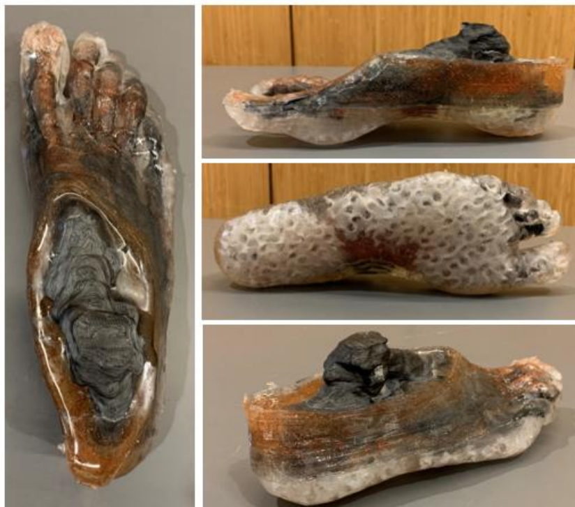
Figure 5-16: ARFUP with gyroid lattice visible through the clear gel.
