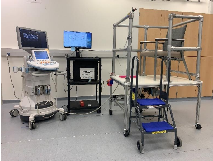
Figure 5-9: The final constructed scanner including both mobile halves secured together, a set of stairs with handles, motors, linear actuators, and DIN rail mounted electrical system, HDPE plate and water bath, and a chair for the subject to sit on during unweighted data collections.
