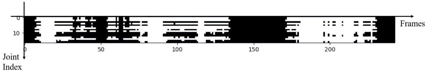
Fig. 6.2. An example of the generated mask in 2D pose estimation. Horizontal and vertical axes represent frame index and joint index, respectively. White color represents the occluded joints while black color represents non-occluded joints.
