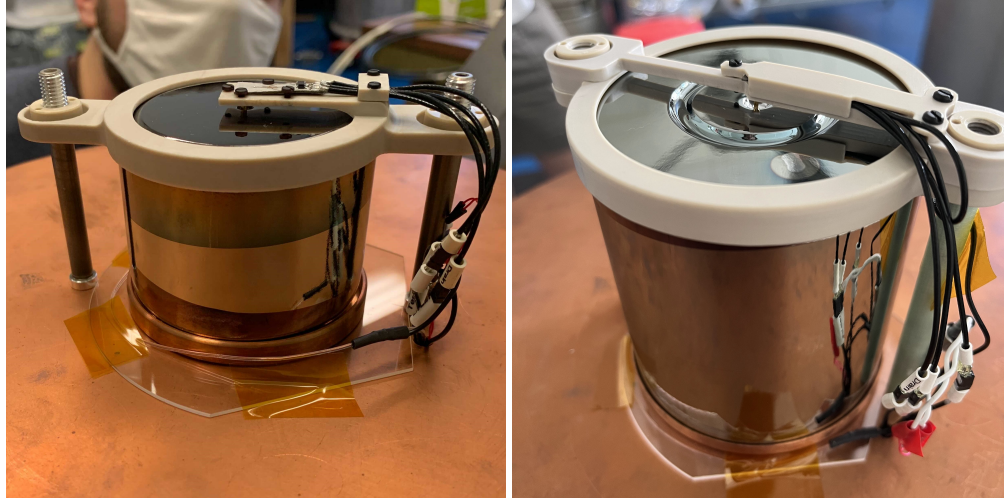
Figure 3.2: Comparison of PEEK support structures for detector and front end electronics board for OPPI ( left ) and ICPC ( right ).
