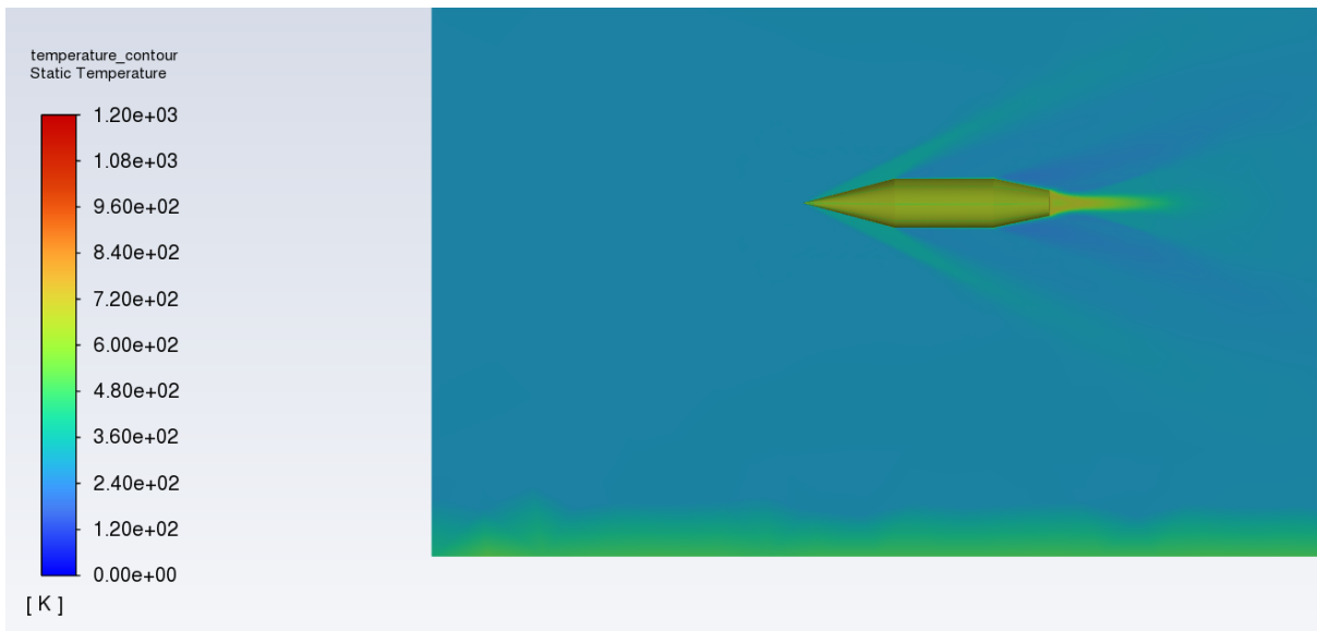
Figure 89. Temperature contour of P380-2BL-12-15 in free flight (methane-air mixture at 300 psi) at 1000 m/s.
