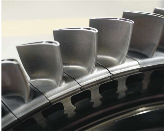
(a) Turbine blade made with metal AM (Siemens)
