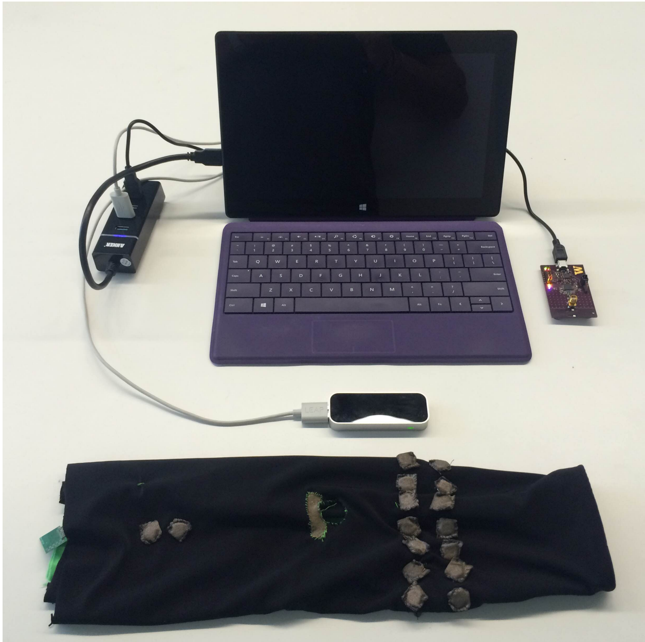
Figure 4.6: Full arm EMG sensing system utilizing custom IC. Sleeve is turned inside out to show EMG electrodes.
