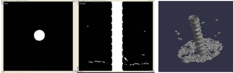
Figure 3.16: Internal Cracking at Load Level 6000 lbs
