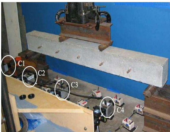
(a) Test Setup with Cameras
