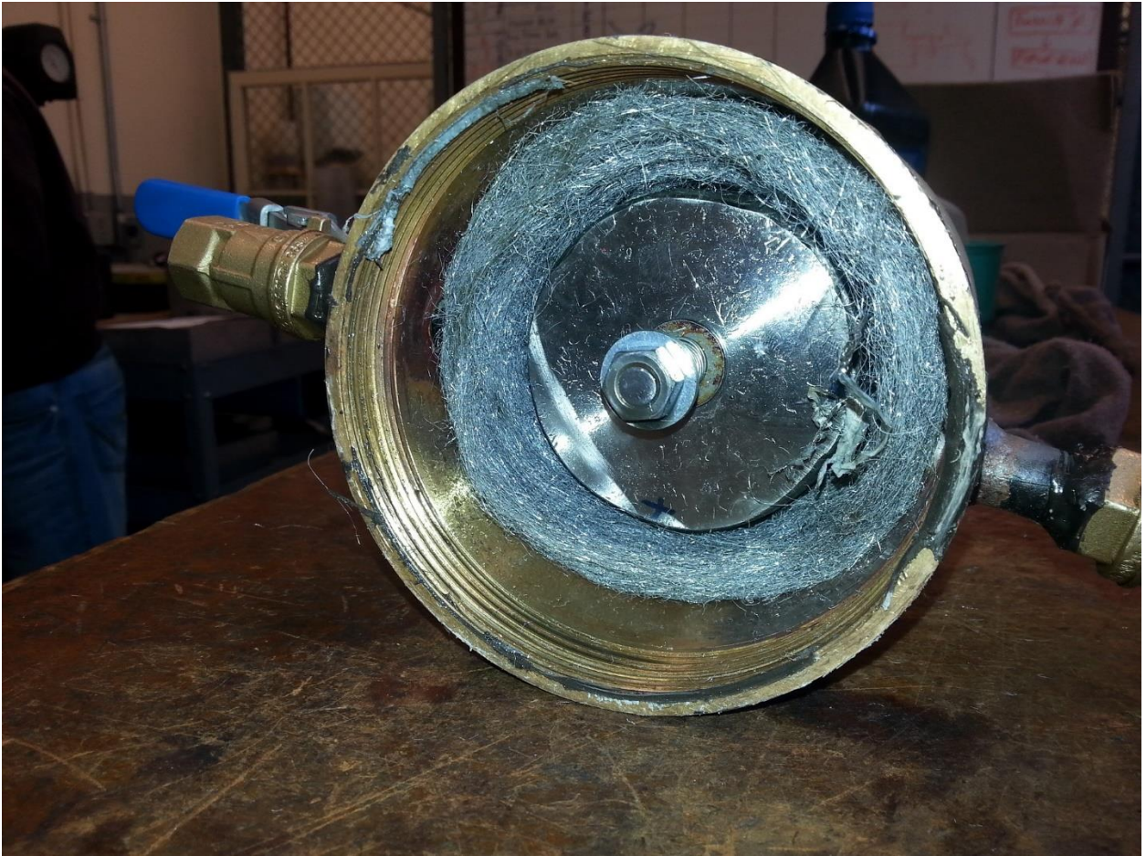
Figure 46: Displacer chamber with regenerator
