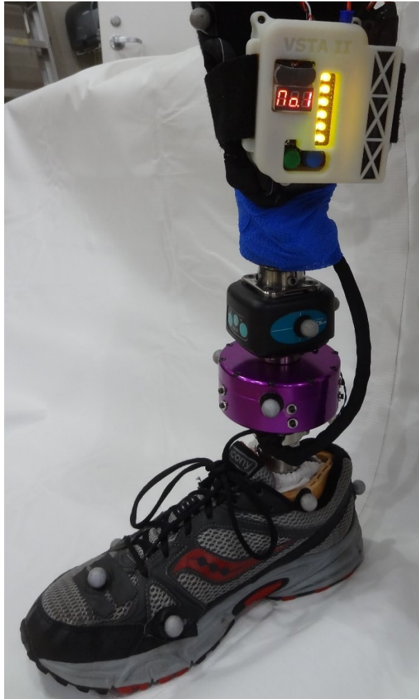
Figure 61: VSTA II installed in pylon of lower limb amputee with iPecs attached axially.
