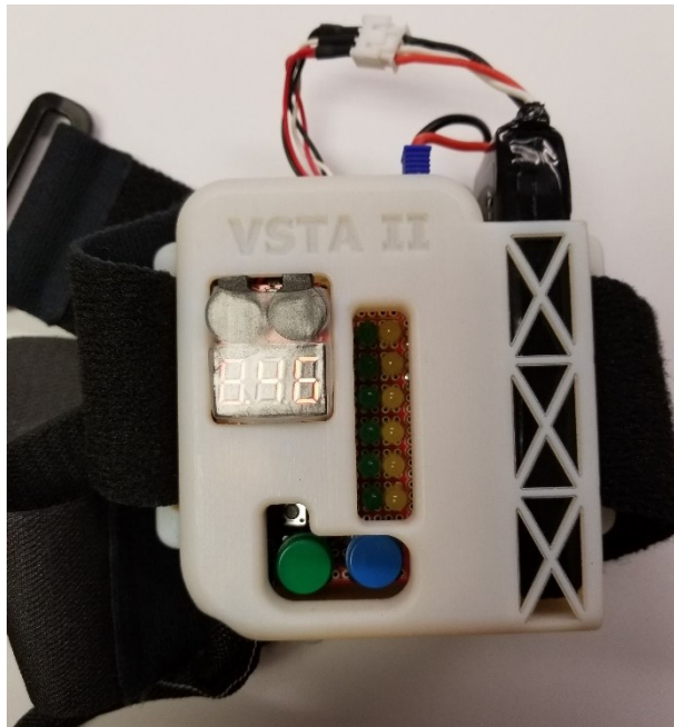
Figure 60: Complete VSTA II controller inside the custom housing with battery attached.
