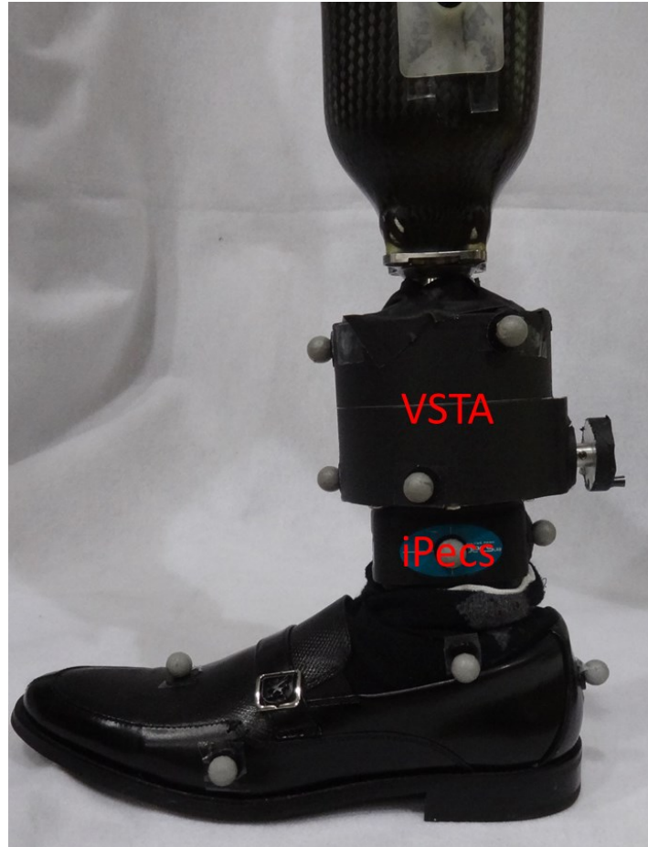
Figure 19: VSTA I setup on VSTA A02 subject with distal installation of iPecs sensor
