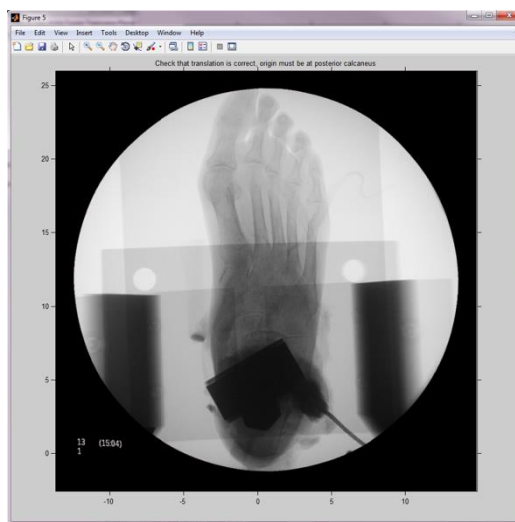
Figure C.9: Check that the most posterior point on the calcaneus is at the origin (0,0).
