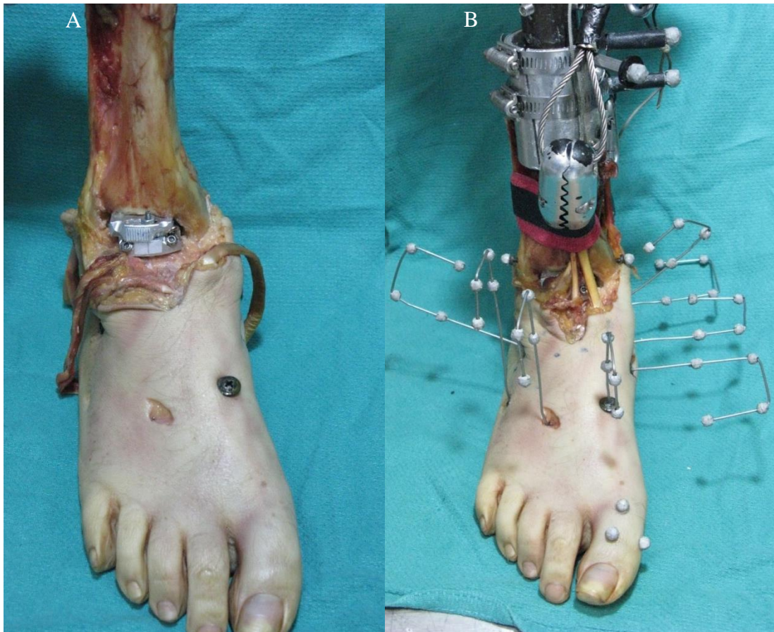
Figure 2.3: A) The fusion misalignment fixture implanted into a specimen showing an internal rotation misaligned position with the tendons dissected proximal to the ankle joint and B) an anterior view of a test specimen, with tendon clamps and strings, Vicon clusters in bone screws, and the tibia mount.
