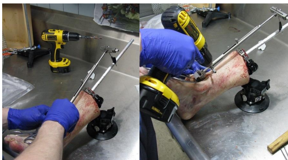
Figure A.4: Placing the alignment guide onto the specimen (left), drilling the pilot hole for the lower pin (right)
