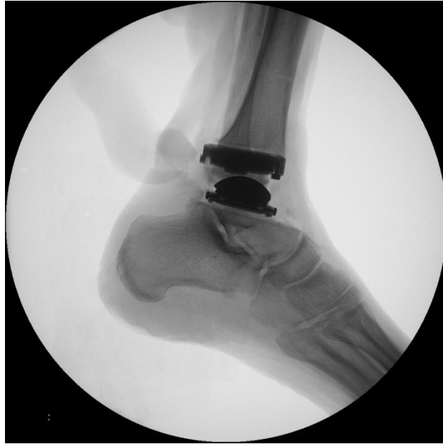
Figure D.22: The implant and fixture assembly inserted into the specimen for alignment, but before fixation.
