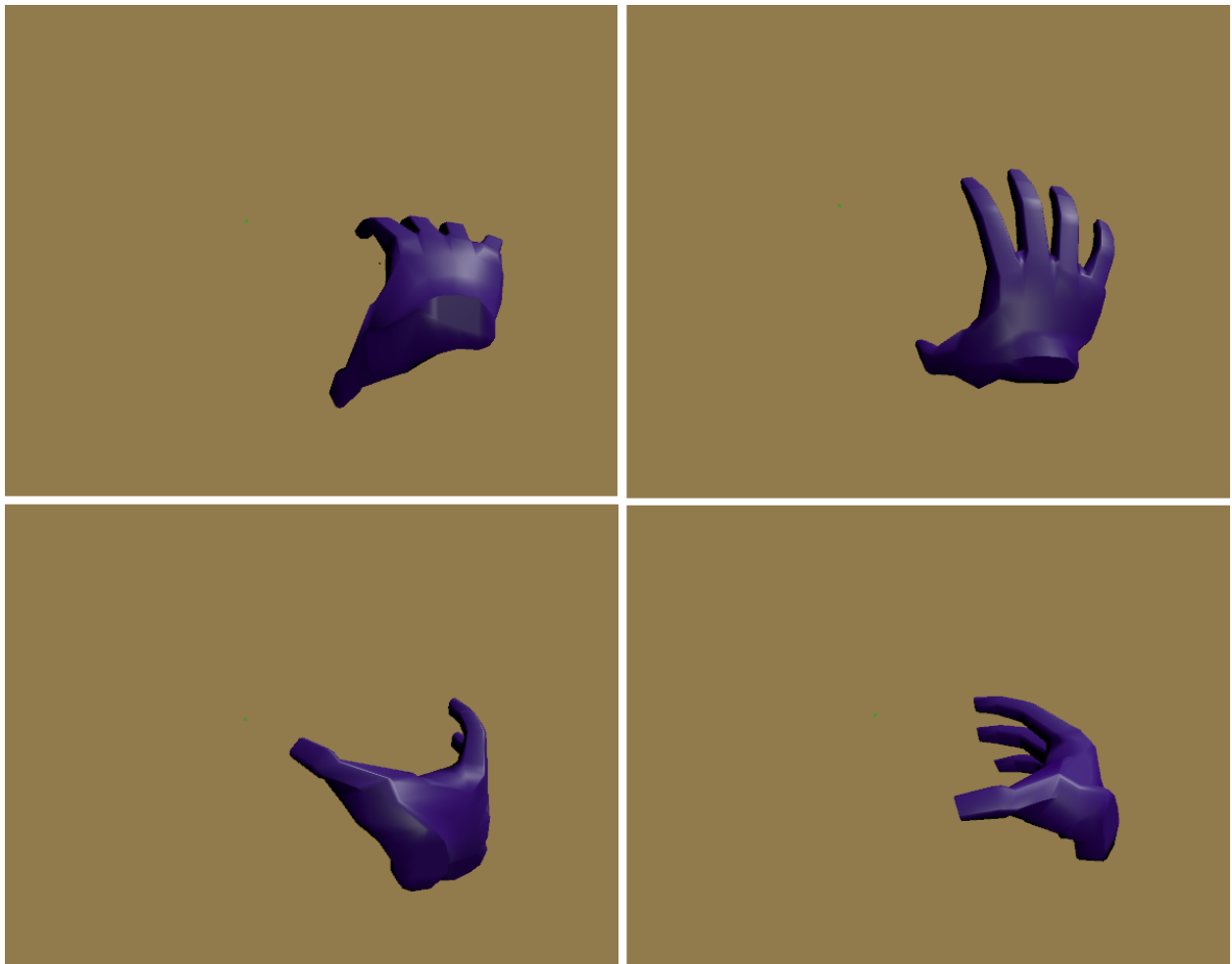
Figure 4.4: Visualization of how each class looks to the user. Each class has a flexion/extension component and a pronation/supination component.
