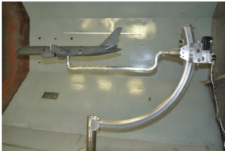
Figure 2.14: 3.5% Scale GTM installed in the NASA Langley 12-ft Low-Speed Wind Tunnel C-sector mounting and positioning system, after Broeren et al. [10]
