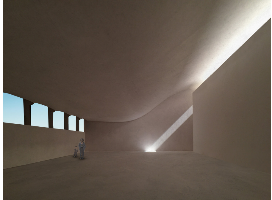
Fig. 119. March/September 21, 12 pm: The light shelf and curved ceiling block all direct light, except for a single beam.
