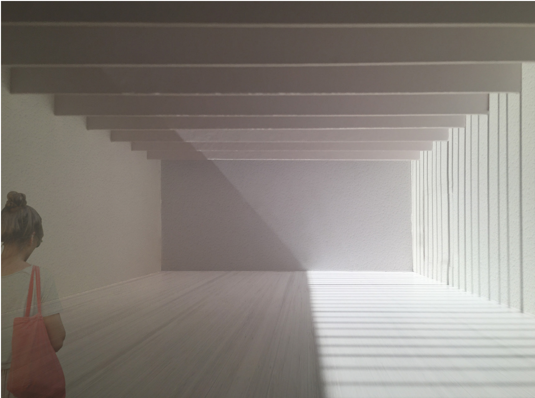
Fig. 132. March/September 21, 12 pm: Stripes of light fall onto the northern wall and floor, while the southern half of the room remains shaded.
