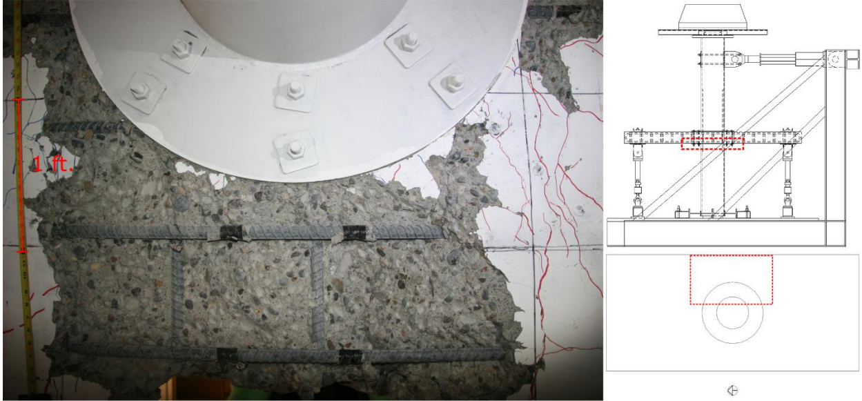
Figure 4-100: Bottom Joint East Side Crushing – 6.4% Drift (PTB_9_2_0)
