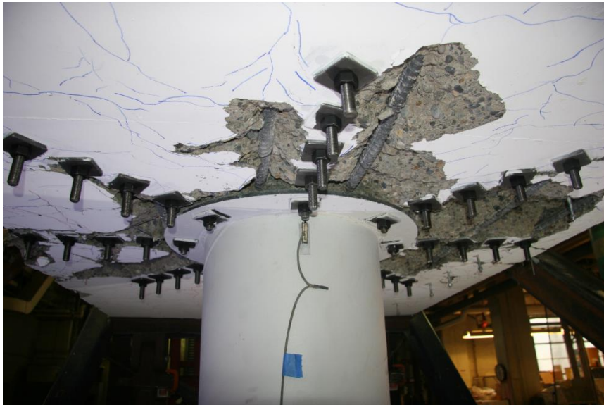
Figure 4-69: Bottom North Side Joint Crushing – 6.7% Drift (PTB_4.5_1_4)
