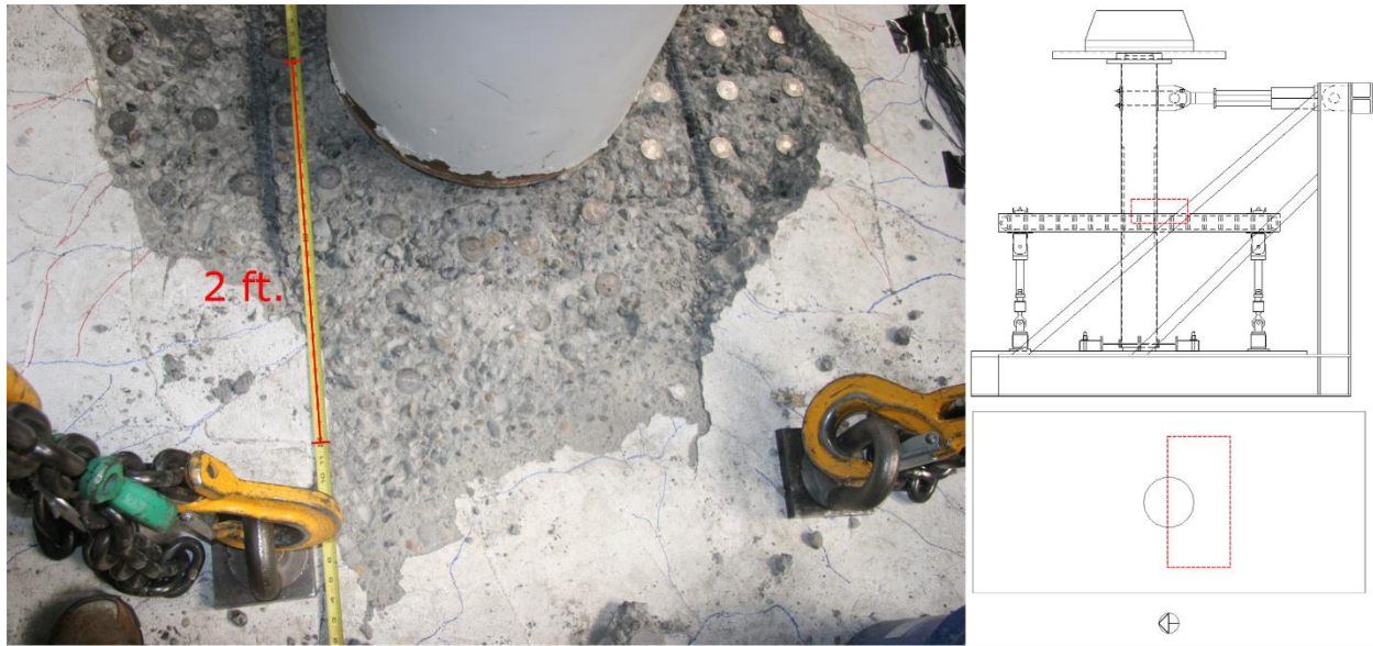
Figure 4-24: Top Joint South Side Crushing – 6.4% Drift (SR_4_10_5)
