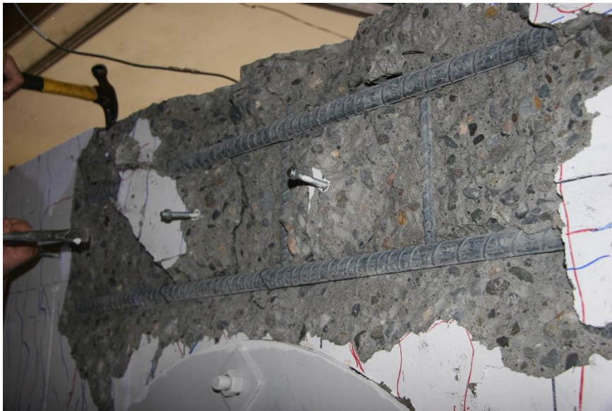
Figure 4-90: Bottom Joint West Side Crushing – 4.9% Drift (PTB_9_2_0)
