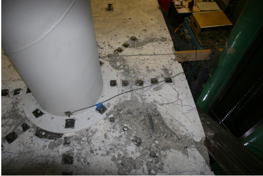
Figure 4-68: Top Southeast Side Joint Crushing – 6.7% Drift (PTB_4.5_1_4)
