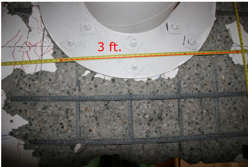
Figure 4-99: Bottom Joint West Side Crushing – 6.4% Drift (PTB_9_2_0)
