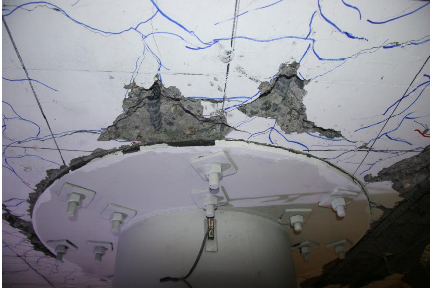
Figure 4-89: Bottom Joint North Side Crushing – 4.9% Drift (PTB_9_2_0)
