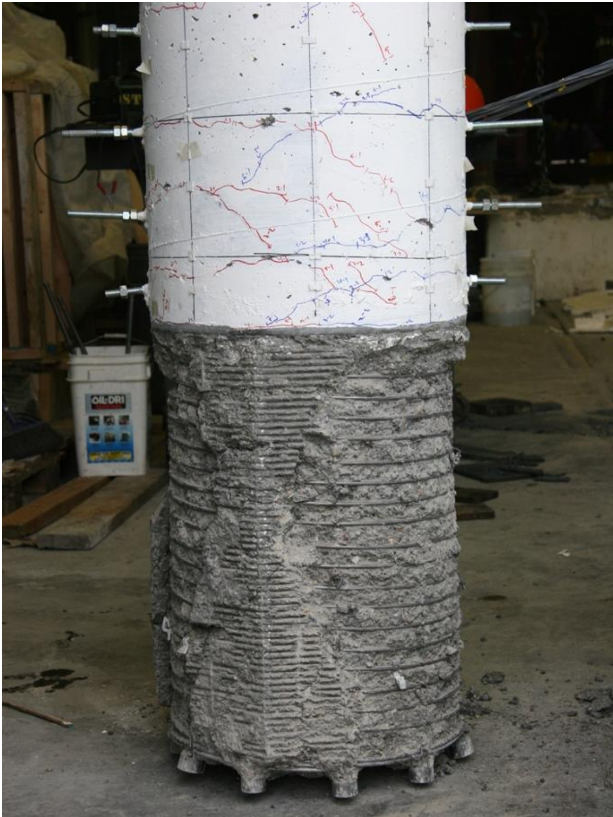
Figure C-0-13. DS-2 – Column damage after cyclic testing
