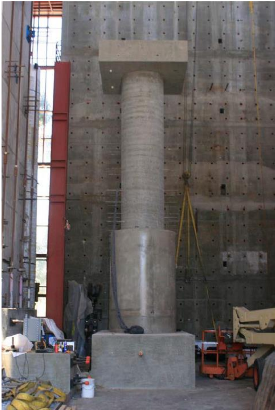
Figure 7-4. Cast-in-place column-shaft connection specimen (Murcia-Delso et al. 2013)
