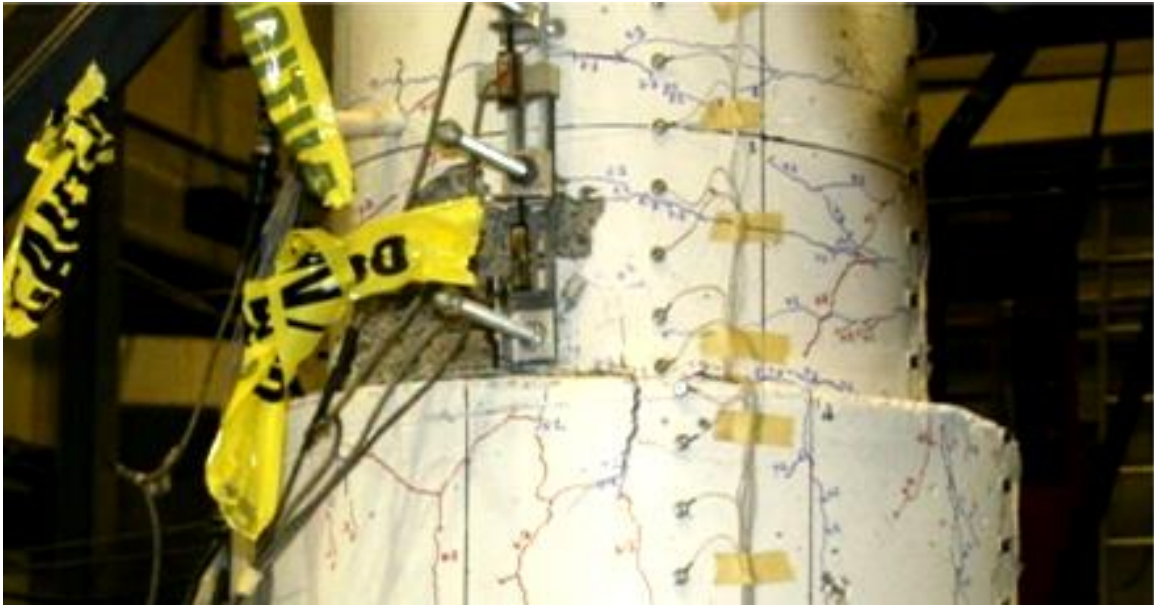
Figure C-0-15. DS-3 – First significant spalling occurred in the column at 2.98/-3.32 percent drift
