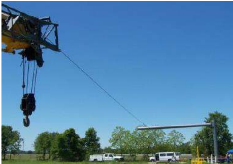
Figure 2.33 Combined torsion and lateral loading (after McVay et al. 2014)
