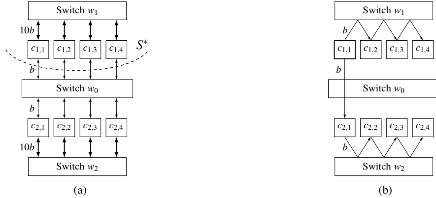
Figure 4.5: Example of Spanning Out-Tree. (a) shows a 2-box 8-compute-node switch topology along with the throughput bottleneck cut. The intra-box connections (thick lines) have 10x the bandwidth of inter-box ones (thin lines). (b) shows one example of ForestColl’s spanning out-trees rooted at c_{1,1} .
