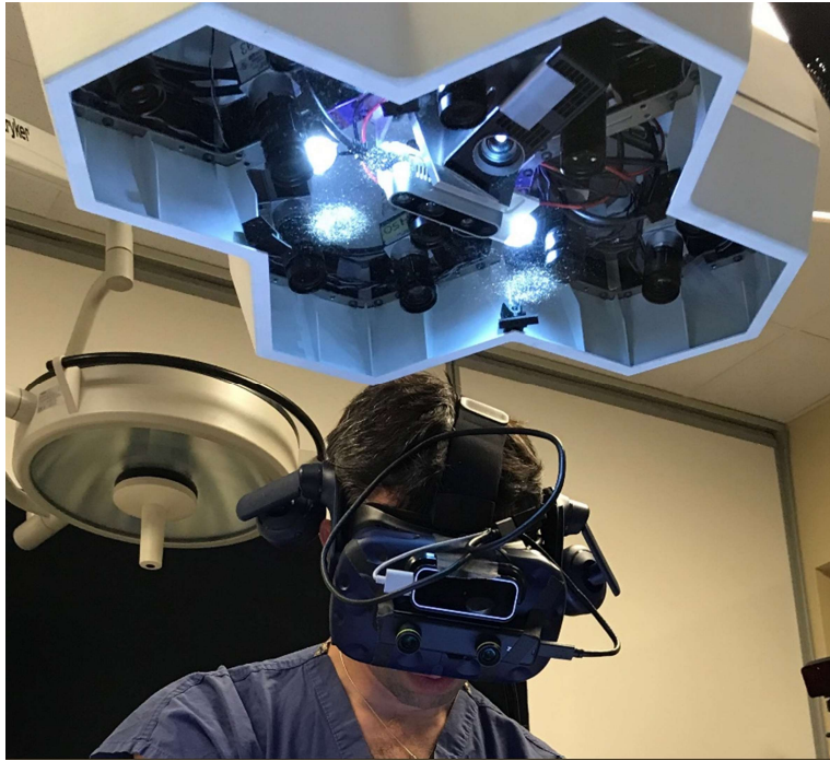
Figure 1.2: A view from underneath the array, showing the cameras, structured light projector, and a surgeon wearing the head mounted display.
