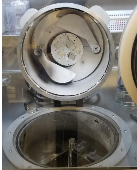
Figure 2.2. Thermal evaporator having the device samples facing downwards to the heated source material which is located at the bottom of the chamber facing upwards. photo from the clean room.
