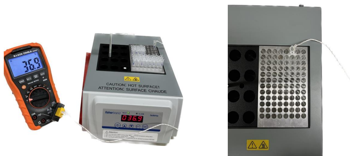
Supplementary Figure 3.16. Machined aluminum plate for cluster tubes (Marsh Tubes, FisherSci Cat No. 07-200-318) in isotemp system.
