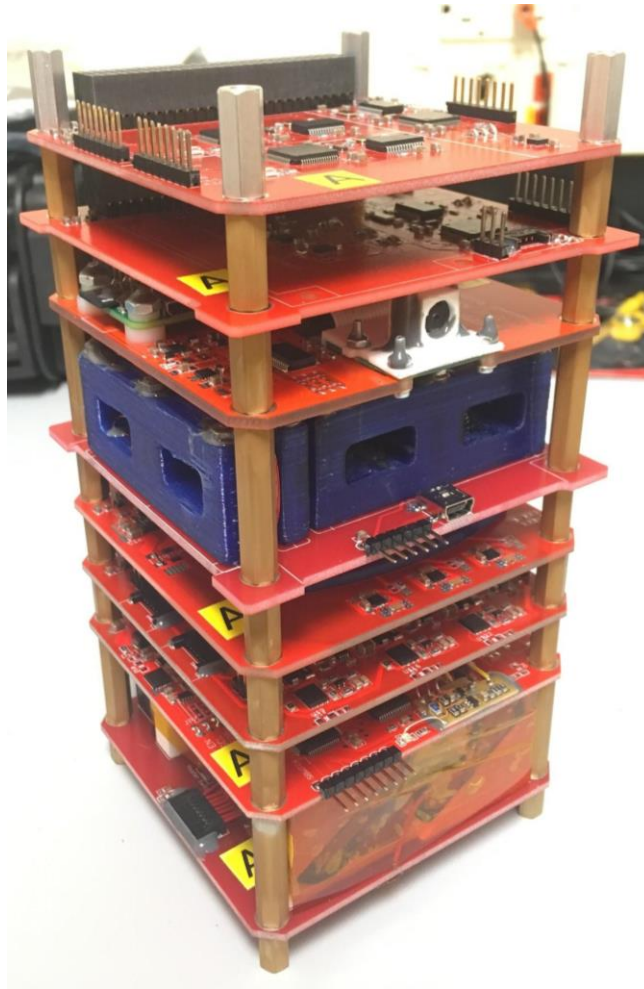
Figure 5.12: Primary Stack (missing COM1)
