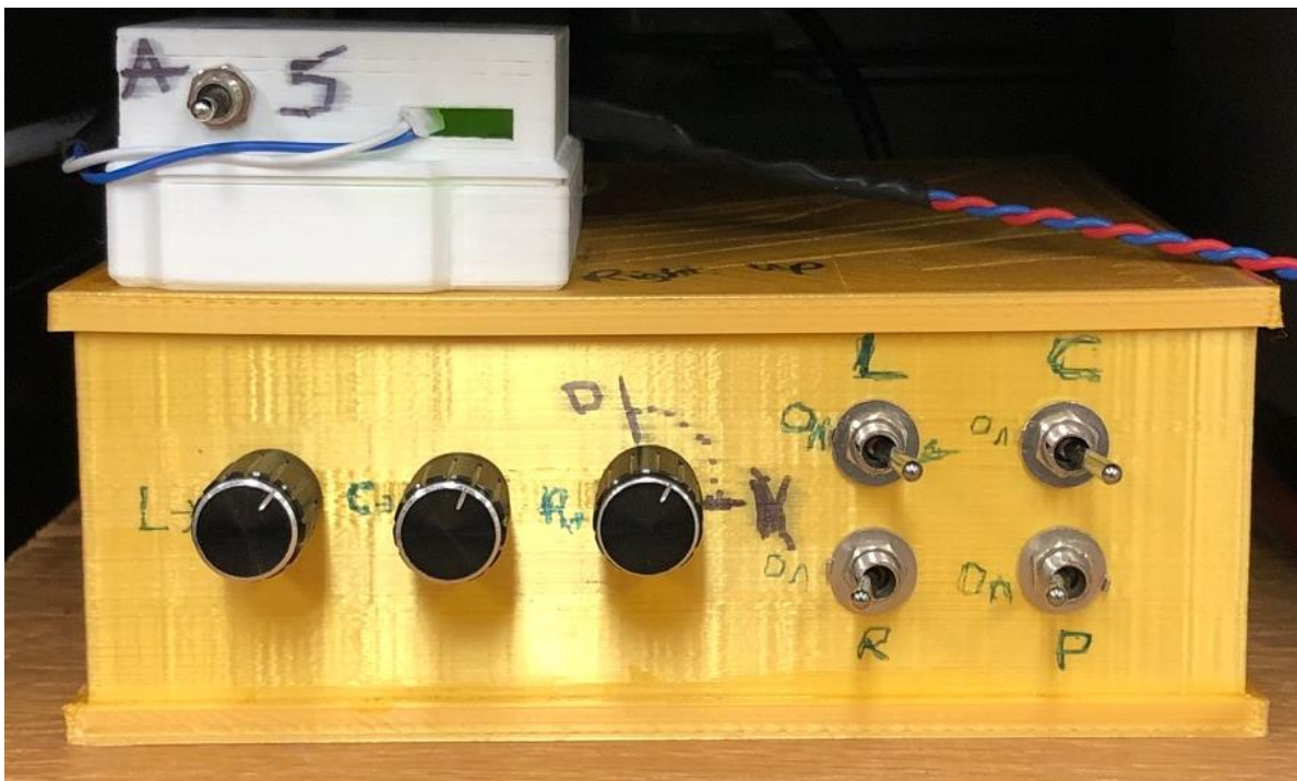
Figure 9: Control unit for arm and filament
