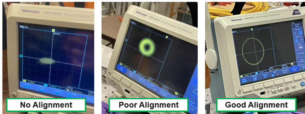
Figure 3.3: Three photographs of oscilloscopes outputting Lissajous figures. From left to right, the figures represent a misaligned chord, a poorly aligned chord, and a properly aligned chord. The misaligned chord shows no circular arc. The poorly aligned chord shows a fuzzy circle of approximately 5 millivolt radius. The properly aligned chord shows a defined circle of approximately 40 millivolt radius.
