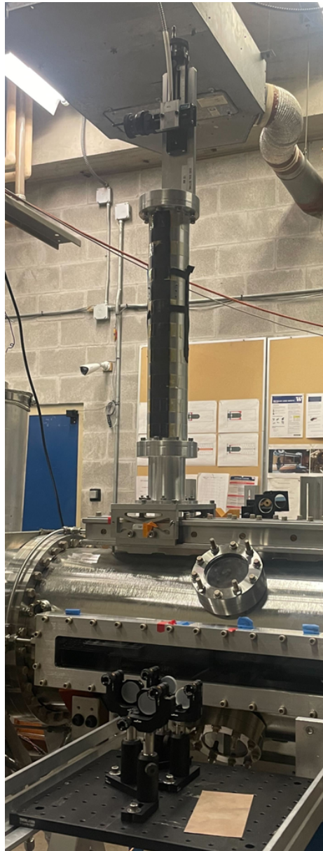
Figure 3.17: Photograph of the radial telescope mounted atop ZaP-HD. It is clear that if the HeNe interferometer is restricted to the typical Mach-Zehnder configuration, that this telescope will block the reference beams. This prevents time-resolved measurements of electron density and ion temperature from being collected in the same location simultaneously.
