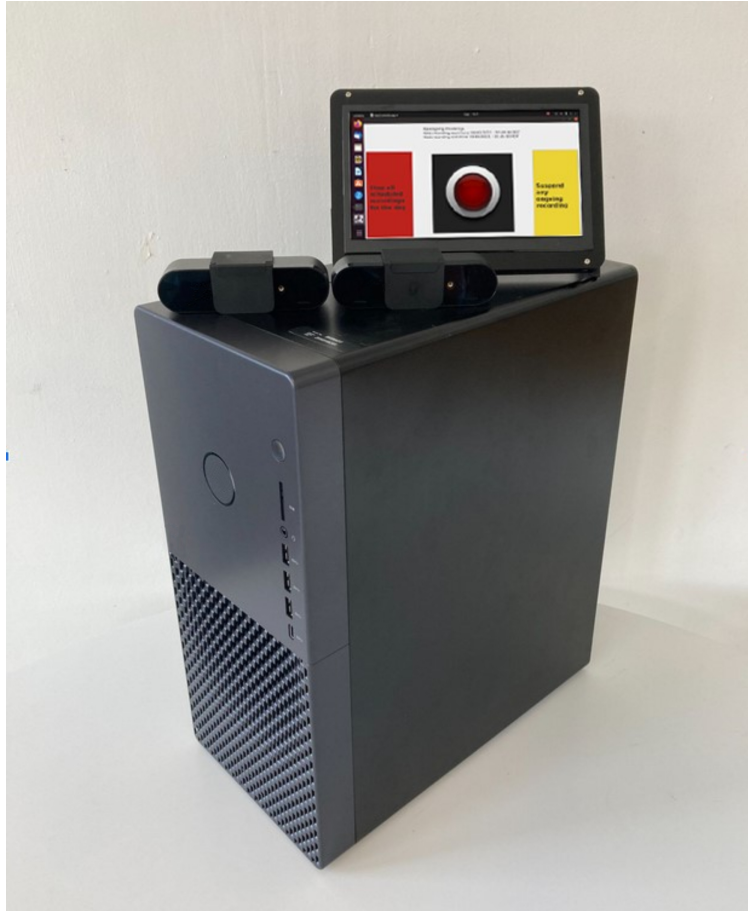
Figure 2.2: Video recording components: The hardware components to support video data collection are minimal, including a single tower PC, USB-connected webcams, and a small monitor to display the patient-facing GUI. The monitor is touchscreen-enabled to allow easy termination of any ongoing or scheduled recordings by pressing the buttons visible on the GUI. The center of the GUI shows an image of a recording light that turns to a bright red color when video cameras are actively recording
