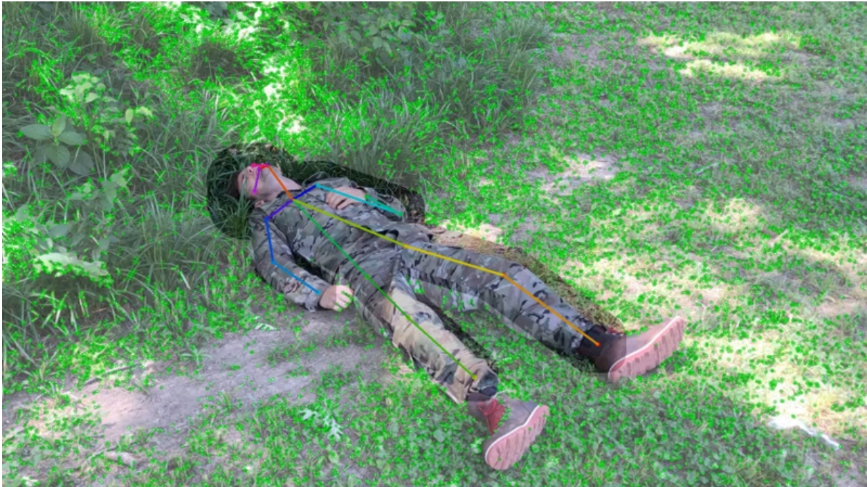
Figure 5.3: This is the demonstration of visual odometry with human motion removed by a mask constructed from the 2D skeleton. The green points are the detected and tracked corner points for VO.
