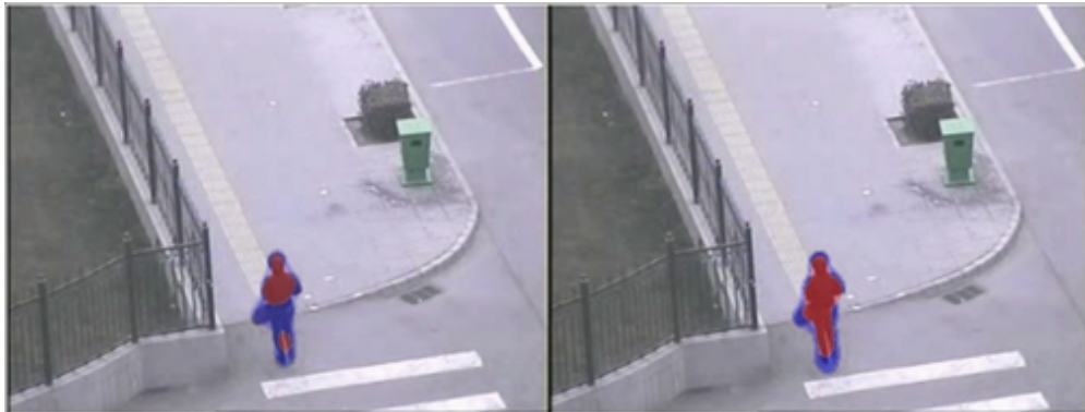
Figure 3.5: This is the comparison of segmentation performance. On the left shows the segmentation from the preliminary results of SuBSENSE with shadow detection. On the right shows the segmentation after the application of multi-kernel feedback loops. Note that foreground is colored in red, and detected shadow in blue.
