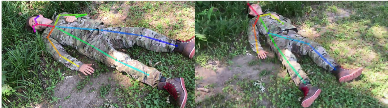
Figure 5.2: This is the demonstration of 2D pose estimation using OpenPose[10], where the 18-point COCO standard is shown on the left, and the 15-point MPI standard on the right.
