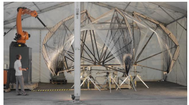
fig. 24 Continuous fabrication of fiber shell
