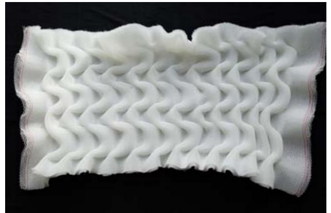
fig. 20 CNC-folded, structural fabric panel
