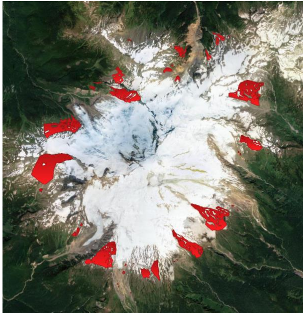
Figure S1. Red polygons show the manually identified static bareground identified on Mount Baker for analysis of the uncertainty of DEMs of Difference (DoDs).
