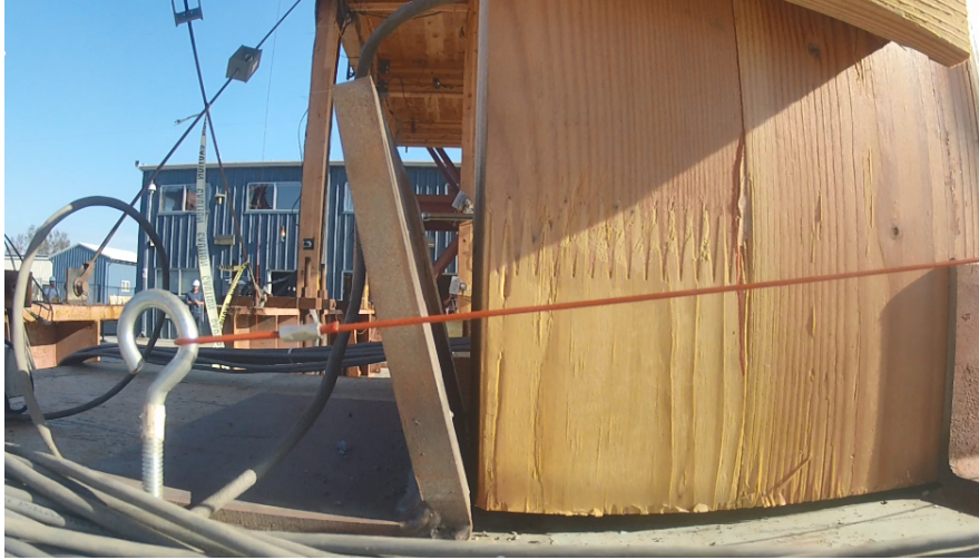
Figure 5.6: Photo showing the gap between the base of the wall panel and the top of the base beam at the end of the testing sequence
