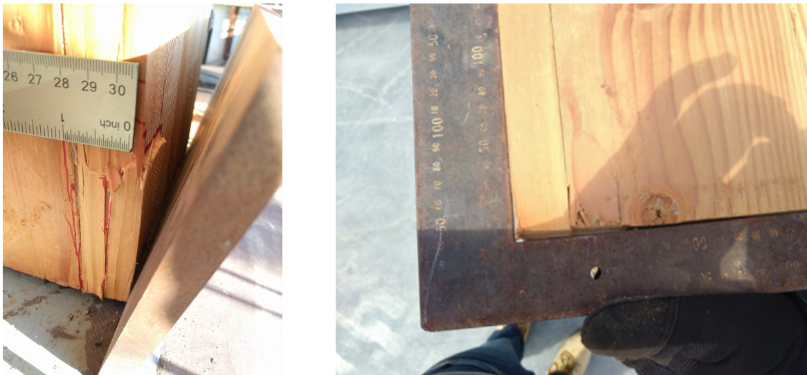
(a) Minimal damage at the corners (b) Minimal permanent deformation to the corners after the walls were removed
