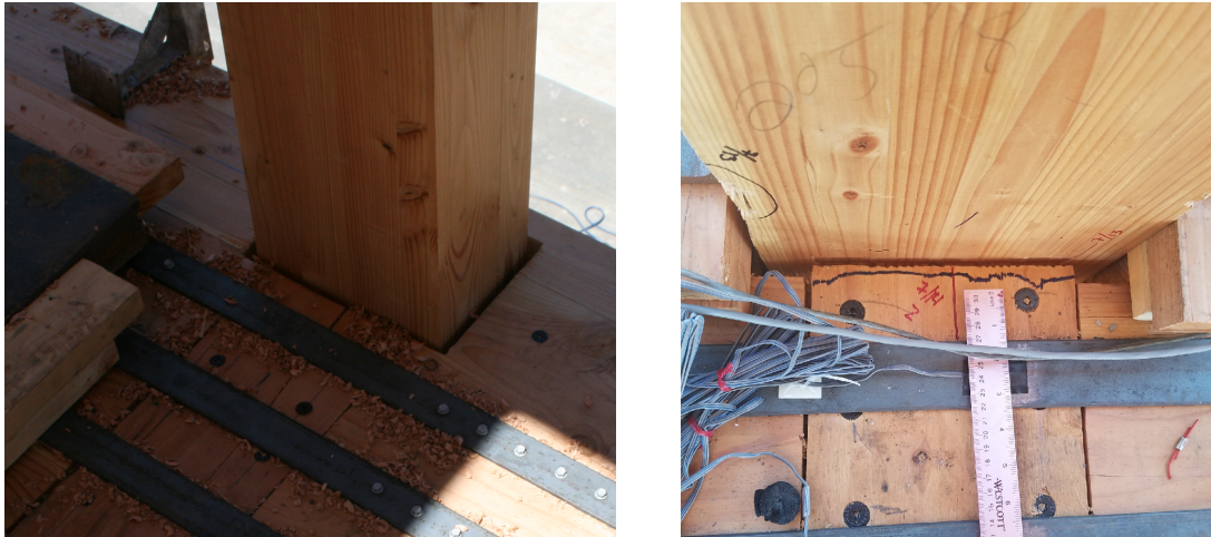
(a) Spline and diaphragm location before testing (b) Spline and diaphragm location after testing
