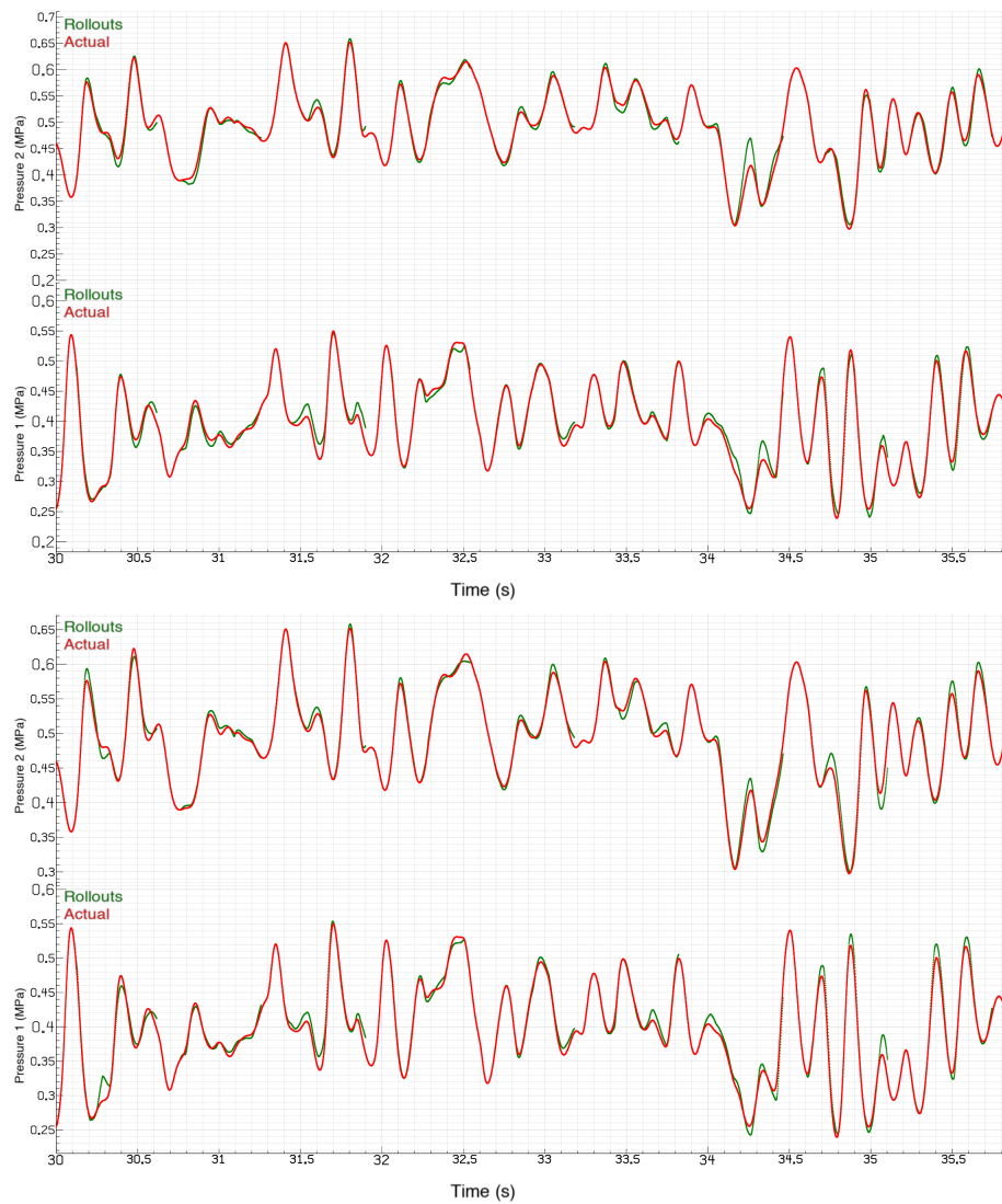
Figure 5.4: Comparison of predicted and actual pressure roll outs for the pure neural network model (top) & hybrid model (bottom)
