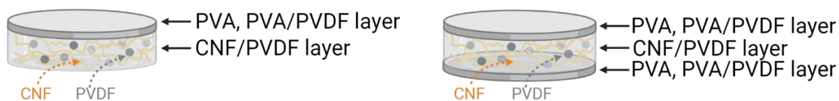
Figure 54. Schematic representing resulting structure of bilayer and sandwich structure films prepared by a film casting process, outlined in detail in the Materials and Methods section of this text.
