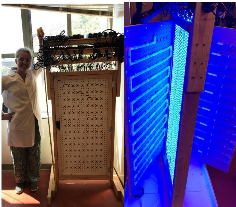
Figure 3.2 : Second generation flow reactor including myself (5' 5'') for scale.
