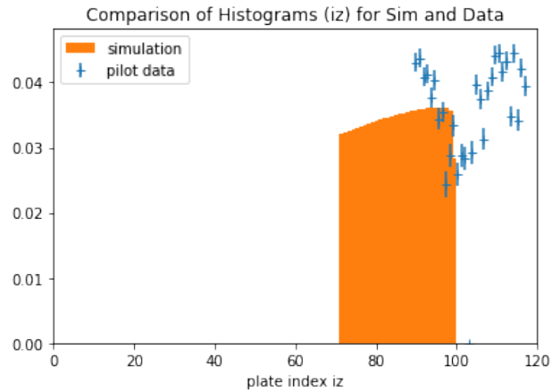
Figure 7.17: Comparison of histograms of iz for simulation (solid color) and pilot data (error bars). The inconsistency does not affect the data/MC comparison, see main text.
