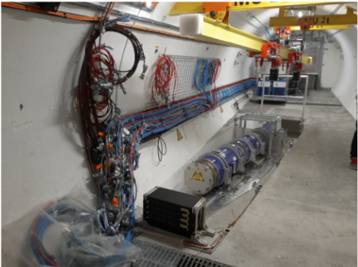
Figure 3.5: FASER spectrometer installed in the TI12 maintenance tunnel of the LHC for commissioning as of 5 February 2021.
