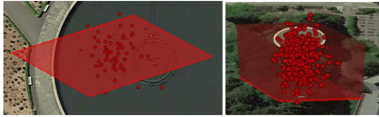
Figure 4.16: ACCV scenario 9, Monte Carlo simulation results top view (left) and side view (right)
