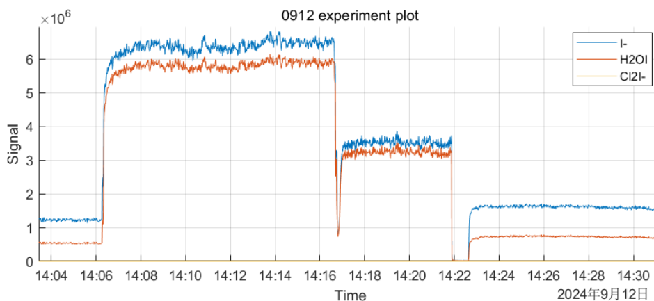
Figure 5. Plot example for the obstructed IMR from nebulization experiments. (14:04~14:06) Full tee gas delivery system attached to the IMR with \text{N}_2 flow sent. (14:06~14:17) Nothing attached to the IMR. (14:17~14:22) only the 1" to 1/2" reducer attached to the IMR. (14:22~14:23) Tee gas delivery system attached to the IMR without \text{N}_2 flow sent. (after 14:23) Full tee gas delivery system attached to the IMR with \text{N}_2 flow sent.
