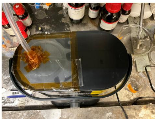
The seal of the nebulizer port (Non-circular port hole)
