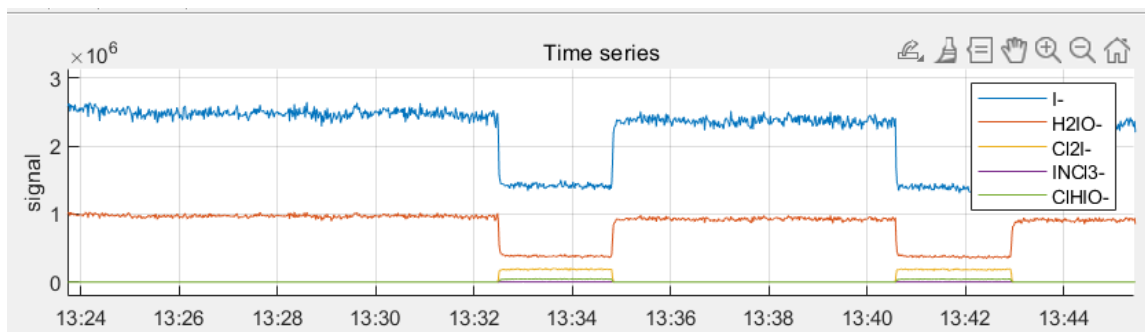
Figure 6. Example for titration. Analytes entering the CIMS would cause the rapid drop of both I^- and IH_2O^- (reagent) and rise of analytes. If the reagent signals dropped too seriously, it means the reagents are titrated.
