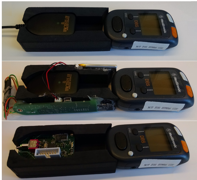
Figure 4.5: The Nexus-D Extension (NexDEx) System Hardware: Top - Normal Nexus-D System. Middle - Prototype Wireless Interface. Bottom - Final NexDEx Implementation.
