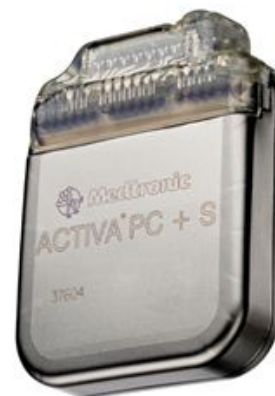
Figure 4.1: The Activa PC+S Implantable Neurostimulator (Credit: Medtronic)
