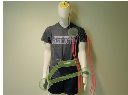
Figure 8.1: A wearable closed-loop DBS system using wearable sensors, smartphone, NexDEX + Nexus-D, and the Activa PC+S.
