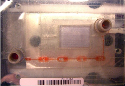
Figure 42 – Recirculation of sample in the microfluidic platform. At time 0, red liquid has been loaded into the pump line, and clear liquid into the imaging chamber (left). Upon starting the execution of the on-card pumps, the sample is recirculated (right). Photo courtesy of Joshua Thompson.
