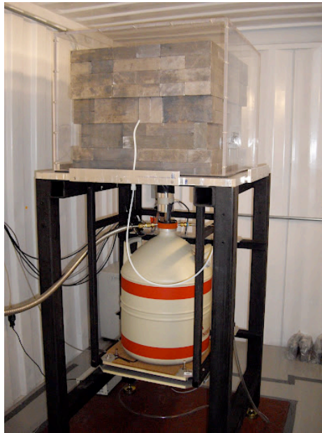
Figure 2.2: The MALBEK detector. The portion of the cryostat containing the germanium crystal is surrounded by lead shielding and a radon exclusion box. The detector is cooled with an LN dewar.
