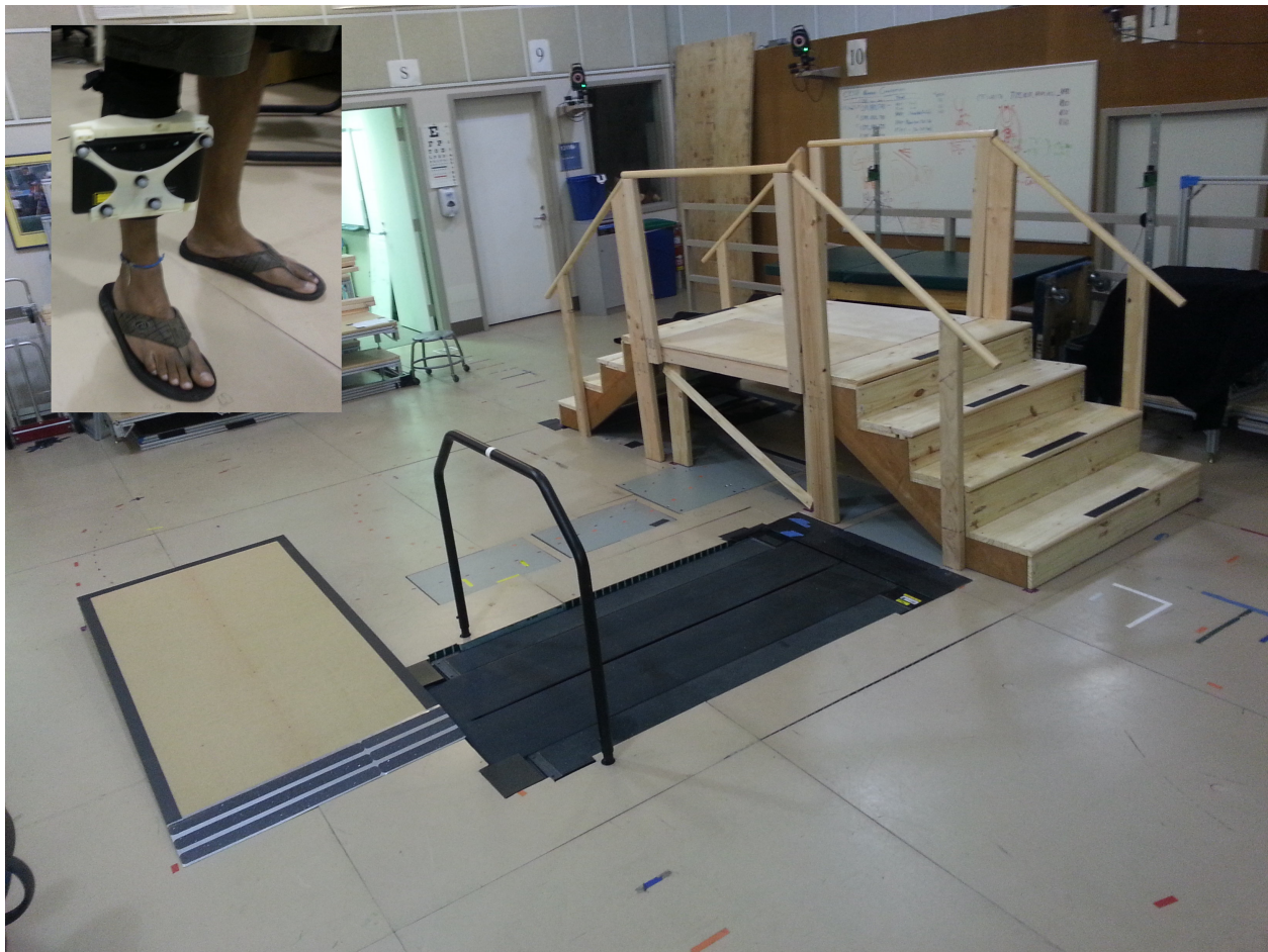
Figure 3.1: Multi terrain course. The 3D-printed mounting frame (inset) integrates with a standard shinguard worn on the shank of the right leg. Participants walked in a rectangular course including up stairs, flat platform, down stairs, flat ground, and a gentle ramp. The black treadmill in the center was not used in the experiment.
