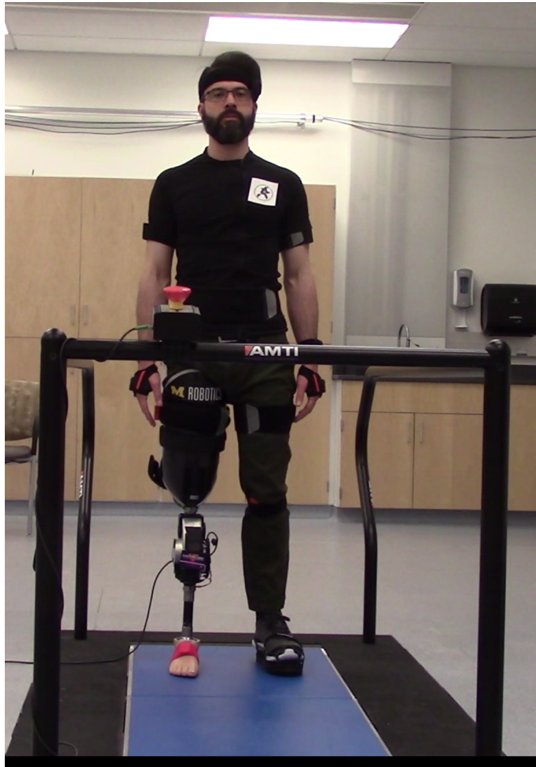
Figure 7.1: Real-time setup with Open Source Leg (OSL). An individual wearing the motion capture sensors walked on the treadmill at self-selected speed. Live kinematics from the suit were used as inputs to a pre-trained network that generated right ankle and knee predictions. These predictions were used to actuate the OSL in real time.
