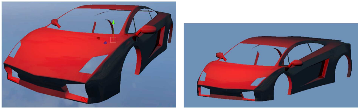
Figure 11. Comparison of images using perspective camera ray generation module (left) and orthographic camera ray generation module (right).
