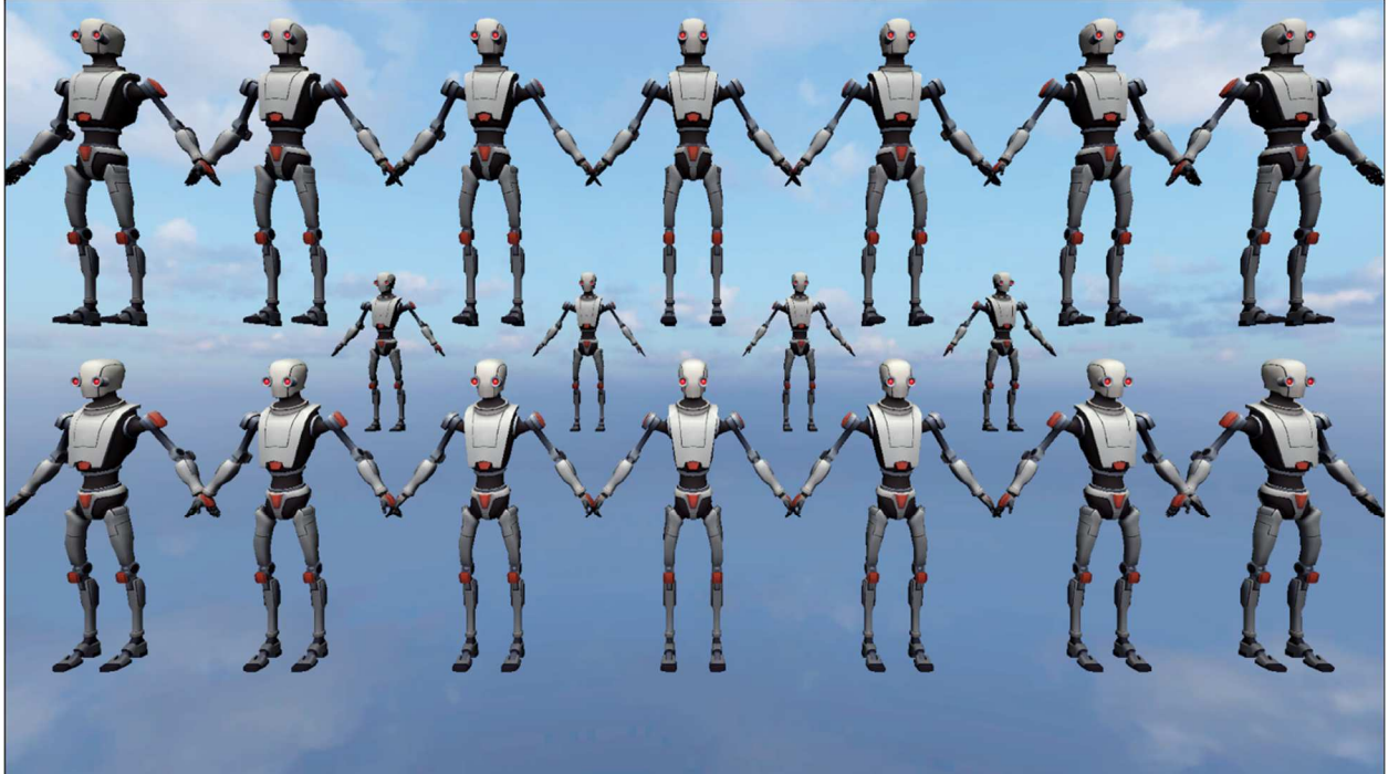
Figure 19. The test scene for measuring the maximum number of triangles supported by our framework. There are more than 104,000 triangles presented in the scene.
