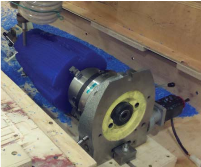
Figure 9: Part and resulting waste after CNC routing
