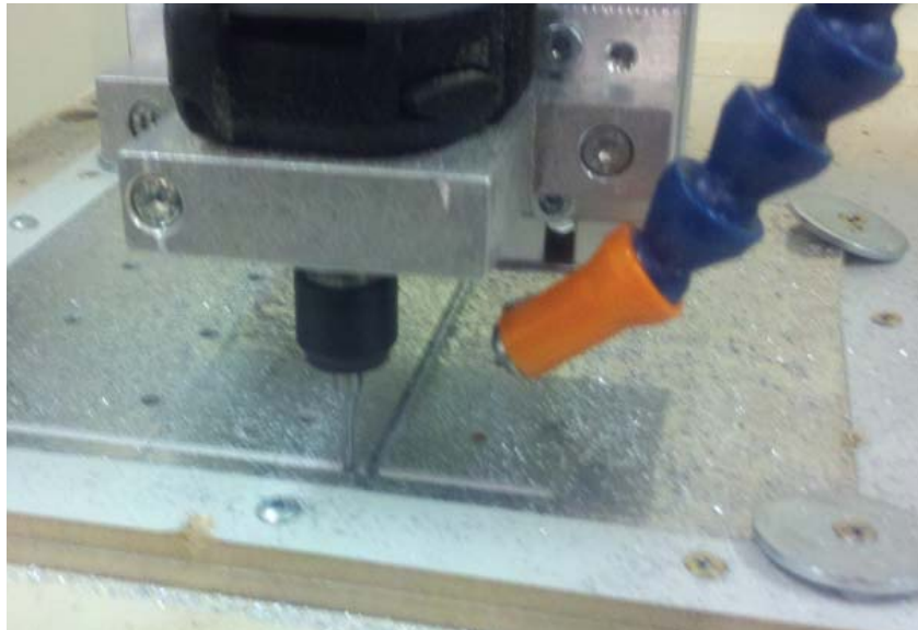
Figure 40: CNC routing fabrication of sheet aluminum wall for final prototype
