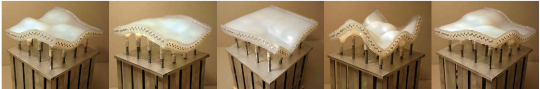
Figure 42: Various mold configurations that [m]form is capable of assuming
