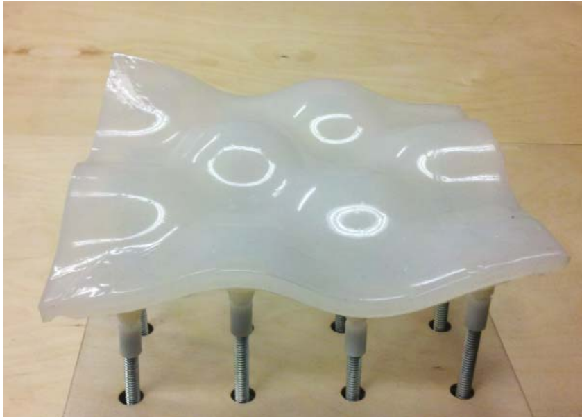
Figure 32: Second [m]form prototype forming membrane and rods
