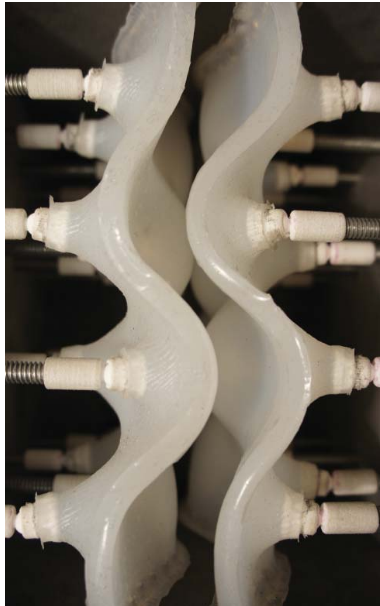
Figure 37: Cast space between two forming membranes
