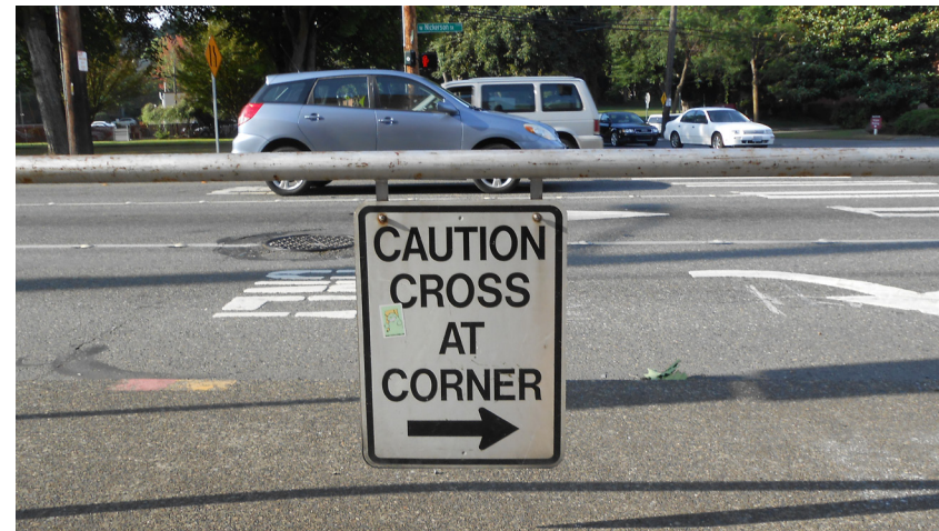
Figure 50 This sign shows the current street crossing problem as the entrance to the rec center is set back from the crosswalk so pedestrians walking the most direct route from campus cut diagonally from the crosswalk and venture into the traffic lanes.
