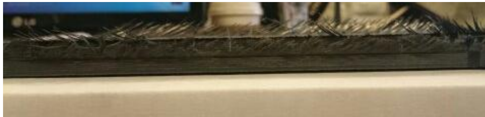
Figure 3.12 : Uni Directional CFRP work piece after Edge trimming , Top view (top), Side view (bottom)
