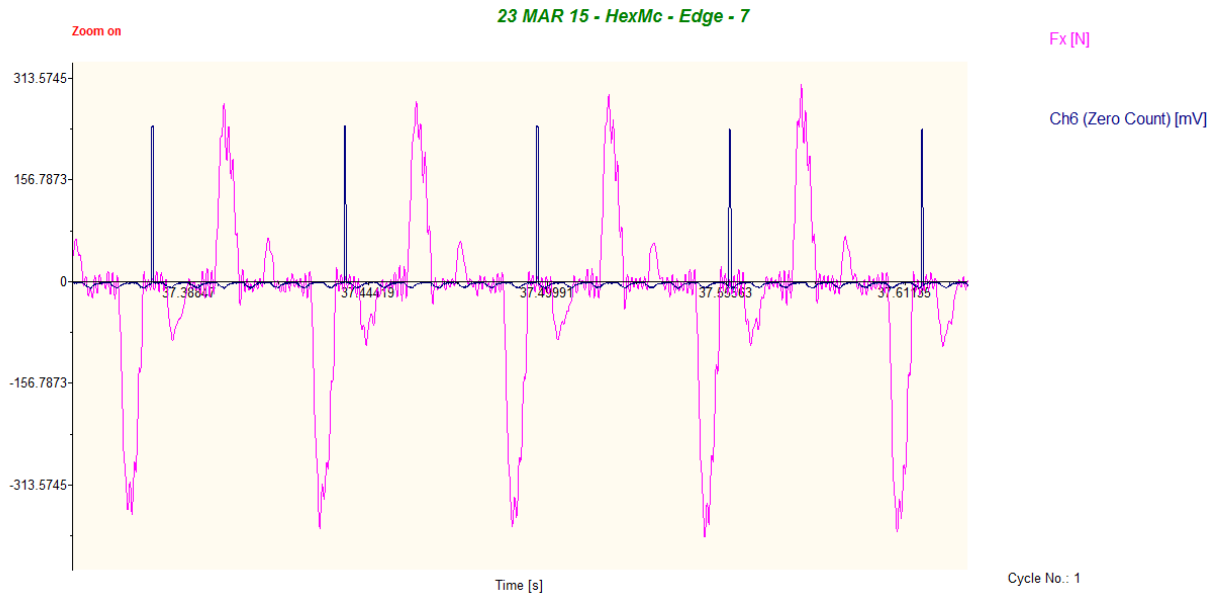
Figure 5.23 : Force and Channel 6 comparison for CFRP and HexMC - Conventional (Odd)
