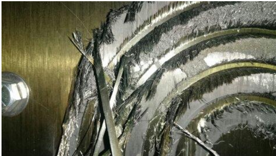
Figure 3.17 : Close up of Circular Slot test - Fiber failure
