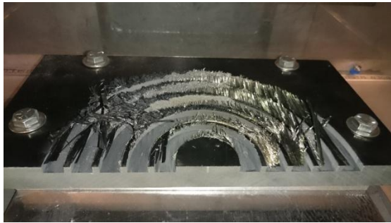
Figure 3.16 : Work Piece after the Circular slot test - before and after dust cleanup (left to right)
