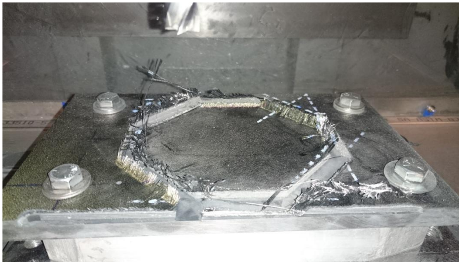
Figure 3.19 : Work Piece after the Octagonal slot test - Top view (top) , Side view (bottom)
