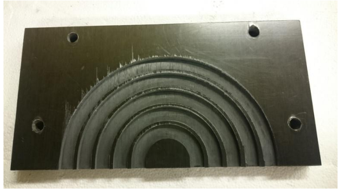
Figure 3.16 : Work Piece after the Circular slot test - before and after dust cleanup (left to right)
