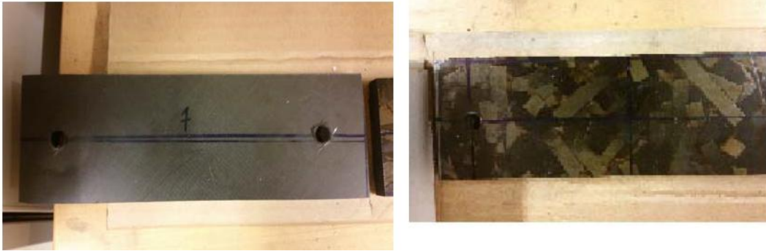
Figure 3.1 : Materials used, Left - UD CFRP, Right - Random fiber HexMC
