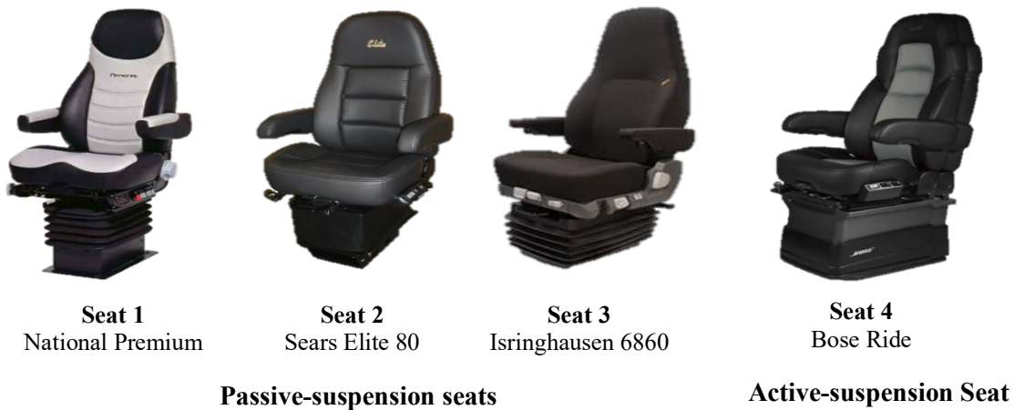
Figure 6 The four seats evaluated in this study: three passive suspension seats, one active suspension seat
