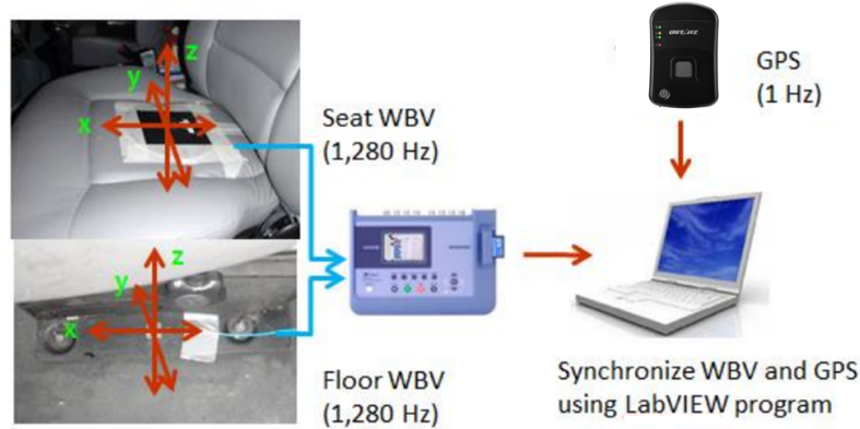
Figure 7 Typical WBV data acquisition set up for this study showing both floor and on-seat mounting of accelerometers
