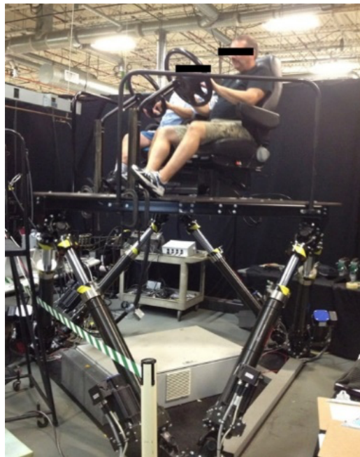
Figure 2 Hexapod mounted with the two truck seats, the active suspension seat is in the background and the passive suspension seat in the foreground
