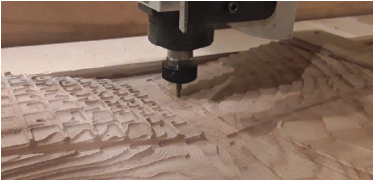
Figure 5.12. Reclaimed English Elm being carved on a CNC router. Creating each model required multiple passes with the tool to refine landscape features.
