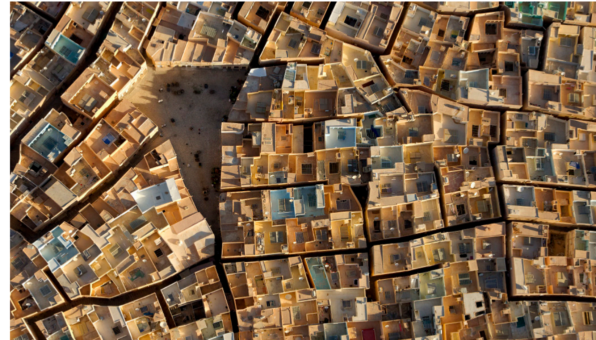
Figure 2.4. An example of a preserved North African hill town's spatial planning and vernacular architecture. Openings in the tops of structures are the impluvia of cisterns for rainwater harvesting. Beni Isguen, Algeria. Source: George Steinmetz (used with permission)
