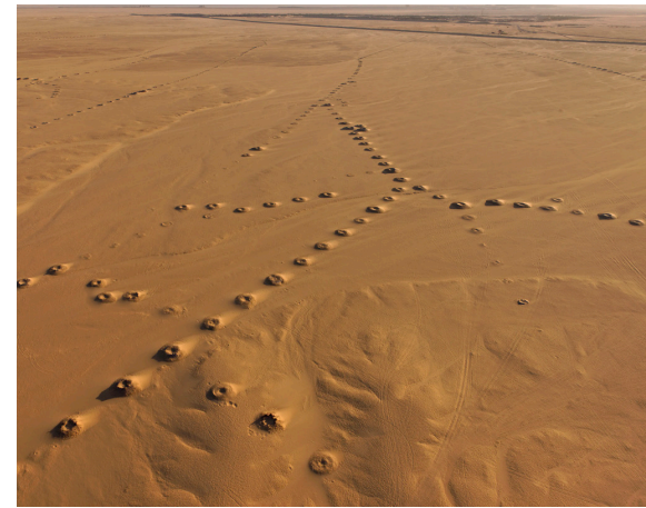
Figure 3.9. Long-distance water conveyance through the desert in the form of mkayel, underground wells that tap into aquifers and daylight in oases. Sahara Desert, Algeria. Source: George Steinmetz.
