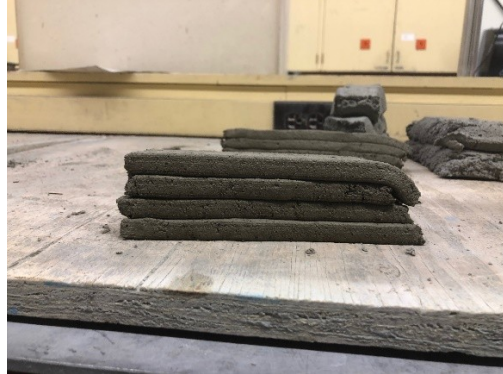
Figure 3.7 0.25 W/C ratio with Walocel
