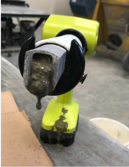
Figure 3.4 Phase migration with sand trials
