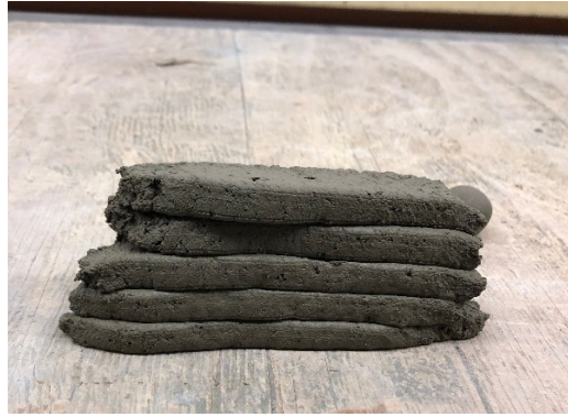
Figure 3.9 0.35 W/C ratio with Walocel
