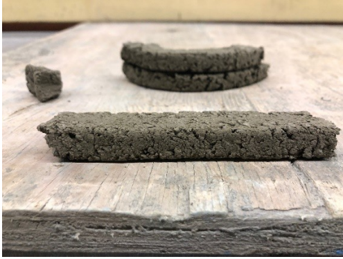
Figure 3.6 0.20 W/C ratio with Walocel
