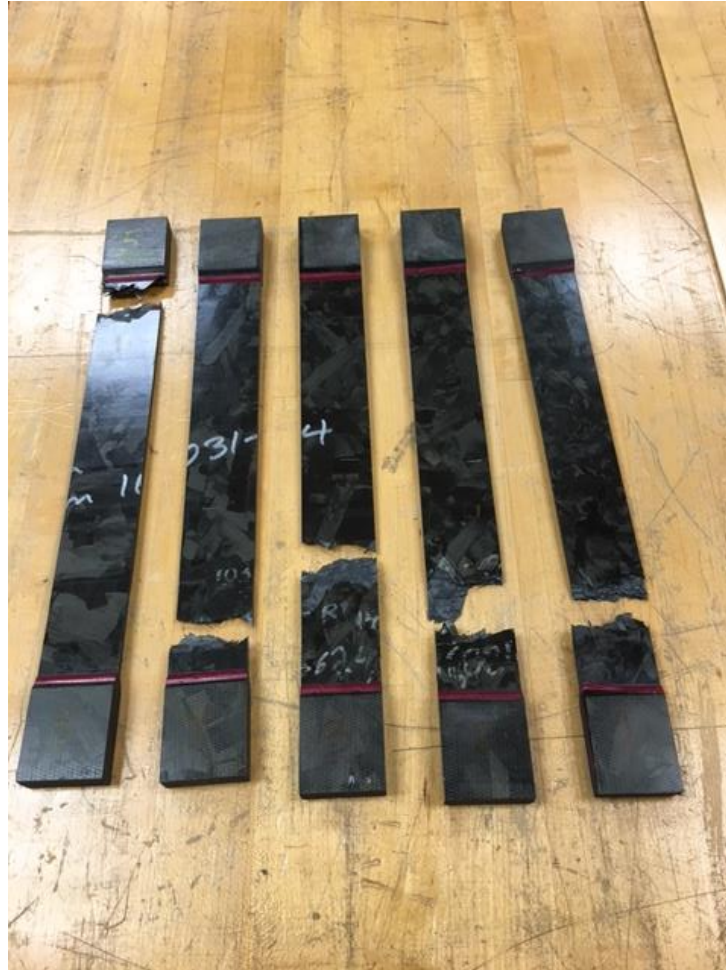
Figure 6.2. Fracture regions of HexMC Flat Panels
