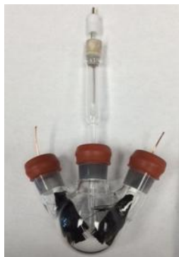
Figure 3.3: Electrochemical cell set up for electro-organic ROMP.
