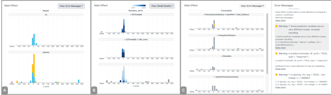
Figure 7-5: A case study illustrating error diagnostics of a multiverse on scientific debate. (a) The Poisson regression model is responsible for all errors, warnings, and abnormal point estimates. (b) Adding random effects greatly improves model quality and removes outlier estimates. (c) A warning of predictors having different scales only occurs in one set of covariates, suggesting the fix of rescaling these covariates.
