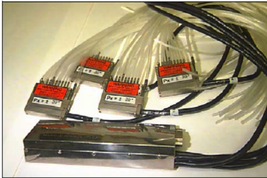
Figure 4.16: Pressure Transducers Used in Pressure Data Gathering
